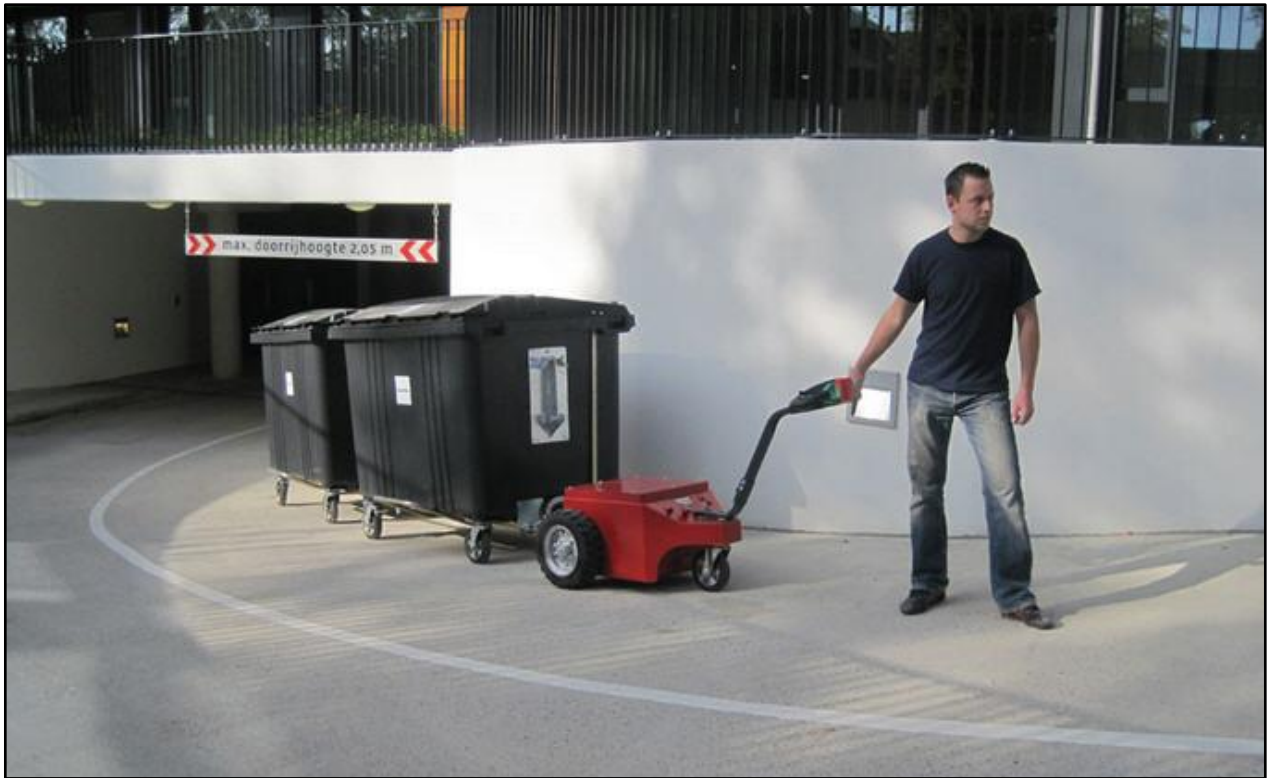
Figure 6: Typical Bin Tug for the 1,100L MGBs
