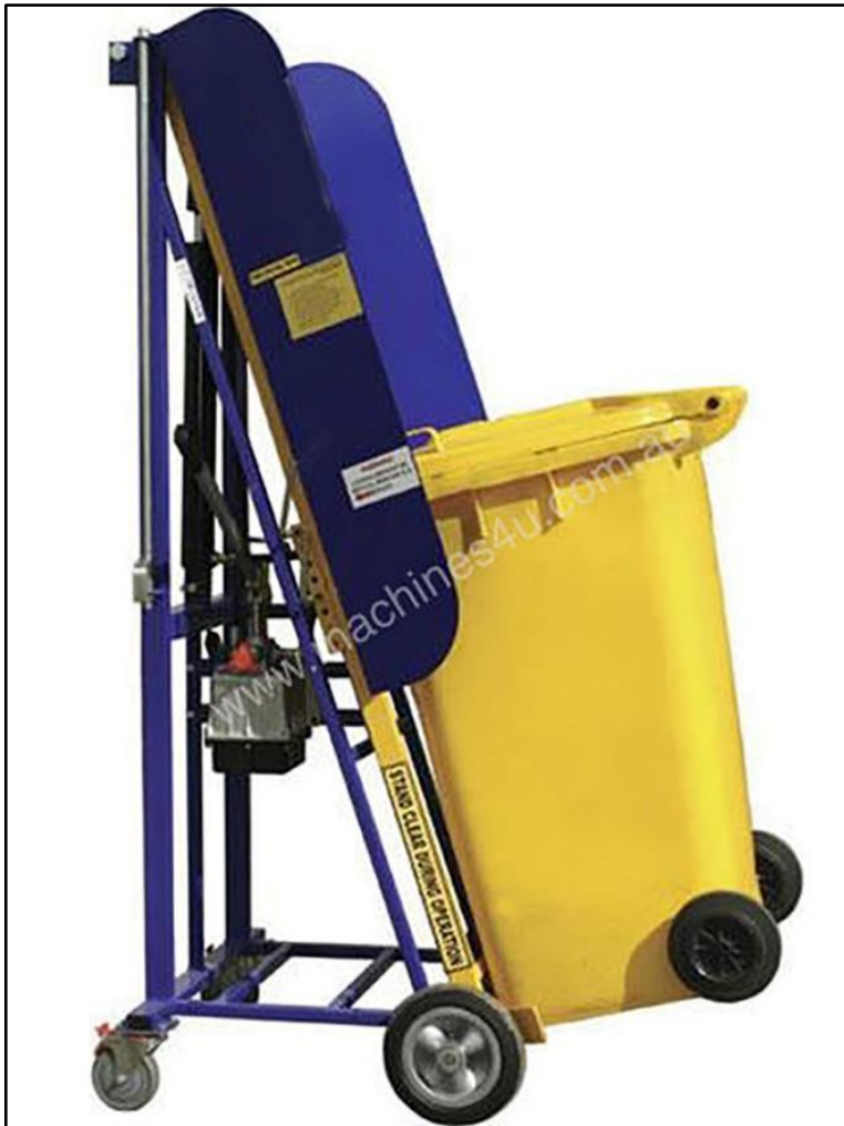
Figure 5: Typical 240L MGB Lift to Empty the MGBs into the 1,100L MGBs
